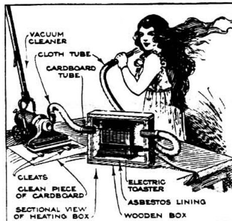
Drying the Hair by Means of Heated Air Furnished by an Electric Toaster and an Electrically Operated Vacuum Cleaner
