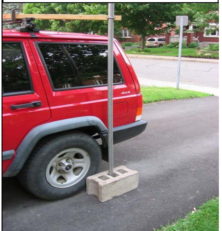
Each 10' mast was clamped to a cross piece and held at the base with a cinder block.
