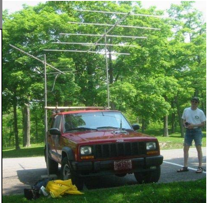
The Ottawa antenna farm. The 2m and 6m beams were installed at different heights to prevent collisions while rotating. A mag mount multiband VHF/UHF antenna can be seen on the hood of the car.
